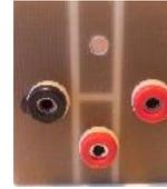
15. Fit the 2mm banana sockets to the DVM PCB. This PCB mounts at the rear of the case using a 3mm x 10mm dome screw, washer, and nut. However you may wish to mount this board to the case after you solder the leads to the board.
