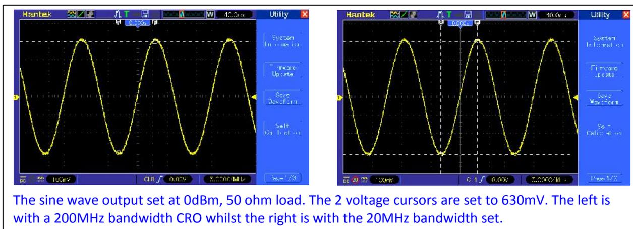
The sine wave output set at 0dBm, 50 ohm load. The 2 voltage cursors are set to 630mV. The left is with a 200MHz bandwidth CRO whilst the right is with the 20MHz bandwidth set.
