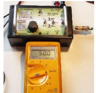
Similarly, switch to -30dBm and adjust that trimpot for 50mV on the DVM.
