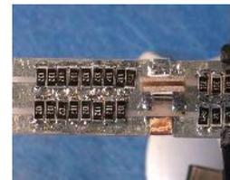
5. Take a piece copper foil as per the video. Cut a square piece which is the width of the PCB. Mark out 2 segments which line up with the earth strips on the PCB and cut as per the video. These 2 narrow strips are soldered to the PCB earth strips at the end of the PCB.
