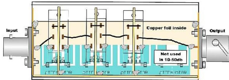
**NOTE:** the 10-50 attenuator uses the 1-10dB case and PCB but only 3 switches are fitted. (this does allow for an additional stage if desired).
