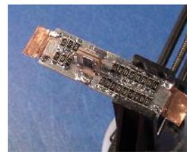
6. Slide the PCB with the foils at each end, into the slots in one half of the metal case. Attach the female end connector to the end of the case using 2 countersunk 3mm short screws. Do not over tighten, and keep straight so as not to cross thread the screw. Do the same at the other end with the other connector.
