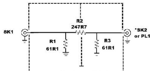
The attenuator is a 50 ohm PI section. The calculated values for 20dB attenuation are:  $R1 = 61.11 \Omega$ ,  $R2 = 247.5 \Omega$ , and  $R3 = 61.11 \Omega$ .
