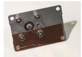
7. Fix a short piece of copper foil to each end plate across the lower half of the connector location. This foil will contact the foil in the case section completing the connector flange earth to the case earth.
