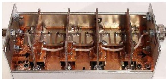
The **ATTN10-50** is a 3 section switchable RF attenuator which provides 10dB steps by selection of various combinations of the 3 sections. The 3 sections are 10dB, and 2 equal sections of 20dB. Operating all 3 switches provides 50dB of attenuation. With the simple shielding used, the amount of attenuation in one unit is limited to a maximum of 50dB.
