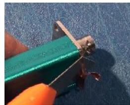
7. Connect the centre conductor of the connectors to the PCB centre tracks using a length of copper wire.
