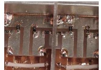
5. With the PCB in a suitable holder, solder the appropriate SMD pad resistors in place in each of the sections on the PCB. Check you have the 10dB resistors on the correct section by laying the PCB in the case over the switch and referring to the label on the front.
