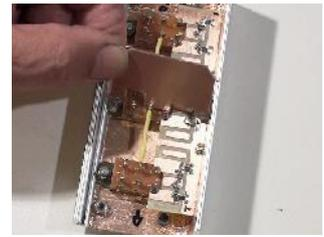
10. Fit the upper case section. That completes the attenuator ready for testing.
